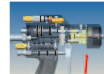
The air piston actuated, gear driven material valve design of the Formula gun has been a part of GlasCraft's gun technology since 1979
